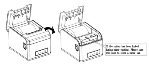
Note: do not force open the cover, as to avoid unrecoverable damage to the print head and the cutter.
