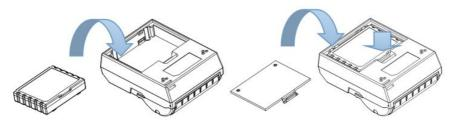
Note: For the first use of the battery, need to charge it full. After the battery is stored for a long time also need to charge it full, then the battery will achieve the best use effect.
